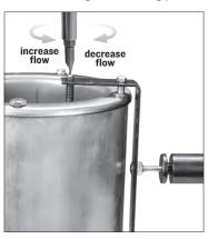
With an ingot mold placed under the pour spout, lift the pour knob and observe the flow. Rotate the valve rod clockwise to decrease flow. As the metal is consumed, you will need to rotate the valve rod counterclockwise to maintain a uniform flow. Do not rotate the valve rod too far counterclockwise as continuous flow will occur. As the valve spout ages, it may corrode or accumulate debris. Should your valve begin to drip,
