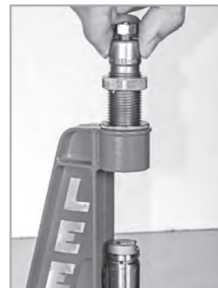
2 INSTALL SIZING DIE If cost is more important than convenience, you can leave the quick change bushing permanently installed after installing the sizing die. While holding the handle against the stop, screw the die in until it touches the shell holder, then release pressure from the handle and screw in the die in additional 1/4 to 1/2 of a turn maximum. Now while holding the die, tighten the lock ring. NOTE: Carbide dies should not be screwed in the additional 1/4 to 1/2 turn.
