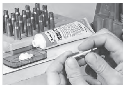
3 PREPARE YOUR CASES Inspect your cases while lubricating them. Discard all cases with split necks, indications of head separation or other defects. Wipe on a thin film of Lee Case Lubricant with your fingers. Fingers are the best way of lubing a case as any grit that could damage the die is wiped away. The case may be immediately sized or you can let the lube dry.
