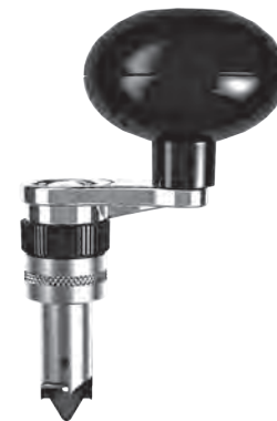
LOCK RING ELIMINATOR Breech lock quick change bushing with integral lock collar provides unmatched precision and convenience when adjusting dies. Split clamp positively locks die into position. 90063 2 Pack
