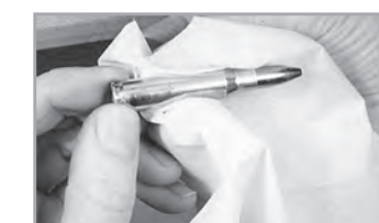
10 IF LOADING maximum loads, it is a good practice to remove all traces of case lubricant with detergent and water. This will reduce pressure against the bolt.
