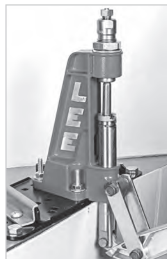
4 PLACE LUBRICATED CASE in the shell holder and raise the ram until the handle comes to a stop. Lower the ram and remove case.
