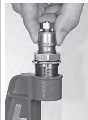
4 PLACE LUBRICATED CASE in the shell holder and raise the ram until the handle comes to a stop. Lower the ram and remove case.
